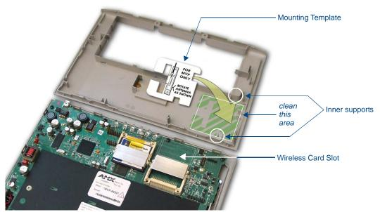
FIG. 10 Installing the Mounting Template
